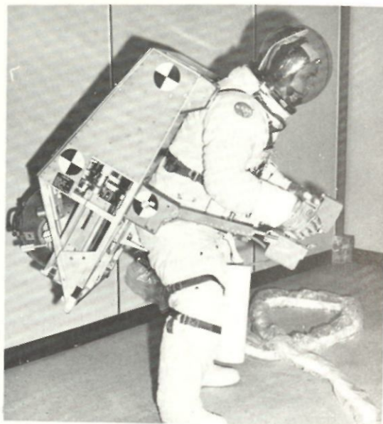
Astronaut Maneuvering Unit backpack, powered by nitrogen gas jets, incorporates four different control systems for flight evaluation in the Workshop.
