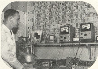
OUTPUT VOLTAGES from nickel-cadmium cells are examined by engineer John Bliven, BSEE, Union College '63 on assignment at G.E.'s Battery Business Section.
