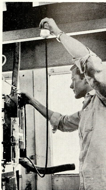
Performing an Orsat analysis of gases by means of chemical actions.
