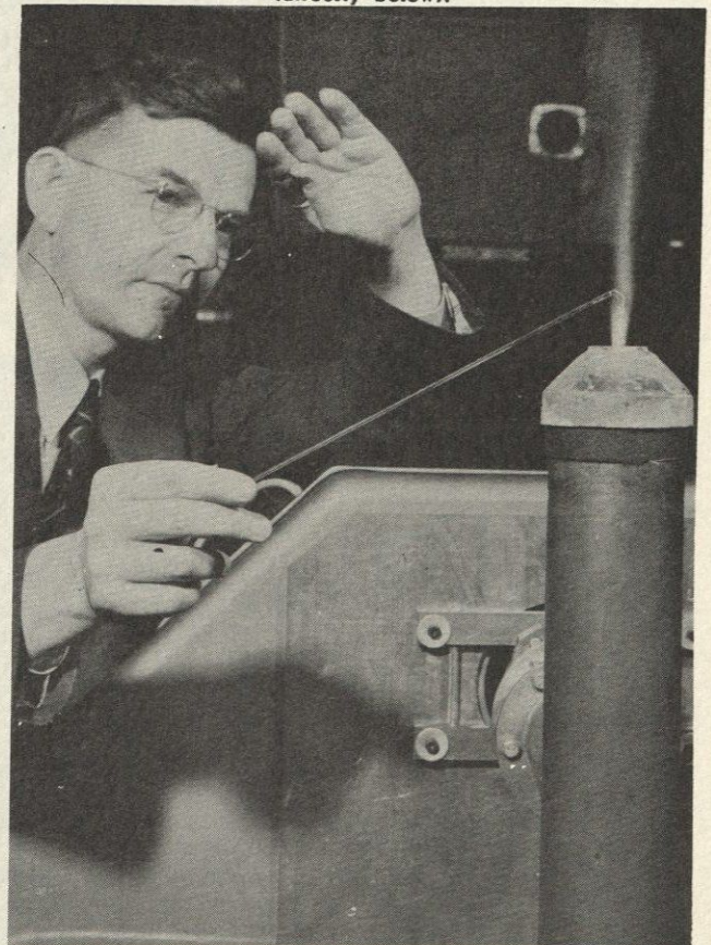
—Courtesy General Electric Co. INDUSTRY. This recently developed electronic torch produces temperatures too high for modern temperature measurement. Quartz (shown), firebrick, and even tungsten melt in the flame consisting of nitrogen passed through a high frequency arc.
