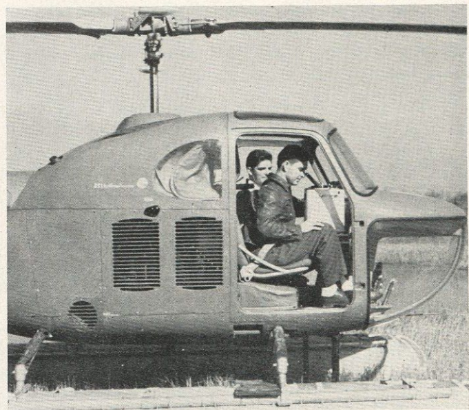
— Courtesy North American Geographical Co. A helicopter equipped with gravity meter facilitates surveys in wilderness regions.
