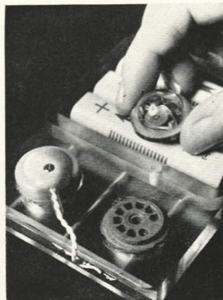
Light telemetry subsystem in which single light-responsive monolithic element delivers an output whose frequency is measure of light intensity.
