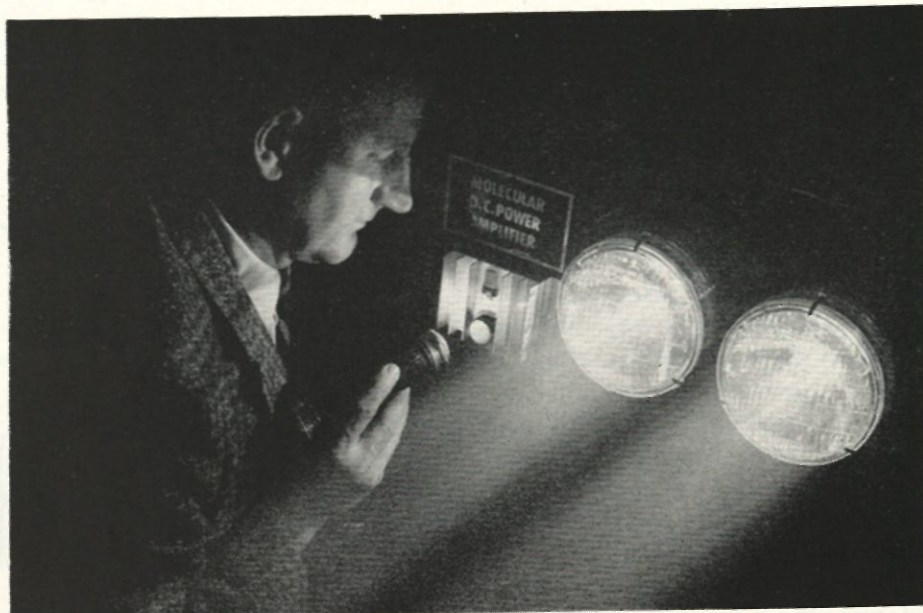
(Not referenced in text.) Demonstration of high-level amplifier as d-c amplifier. Intensity of light impinging on solar cell is fed to function block as d-c signal voltage. Supplied from battery, function block amplifies signal and delivers matching d-c output to head lamps.
