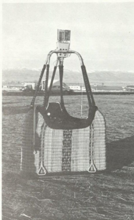
The propane burner sits on top of the basket. The stainless steel coils heat the propane which is vaporized and then burned. Balloonists call this blasting.
