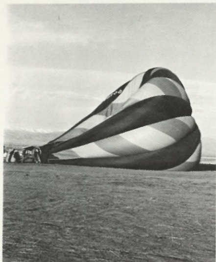
The balloon is about half inflated with cold air.
