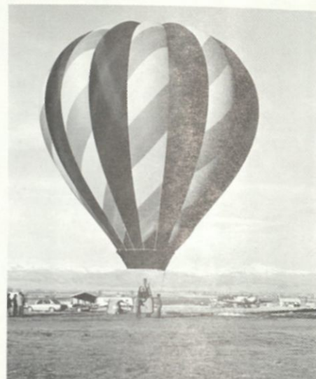
Now fully inflated, the balloon is held to the ground by the weight of the ground crew.
