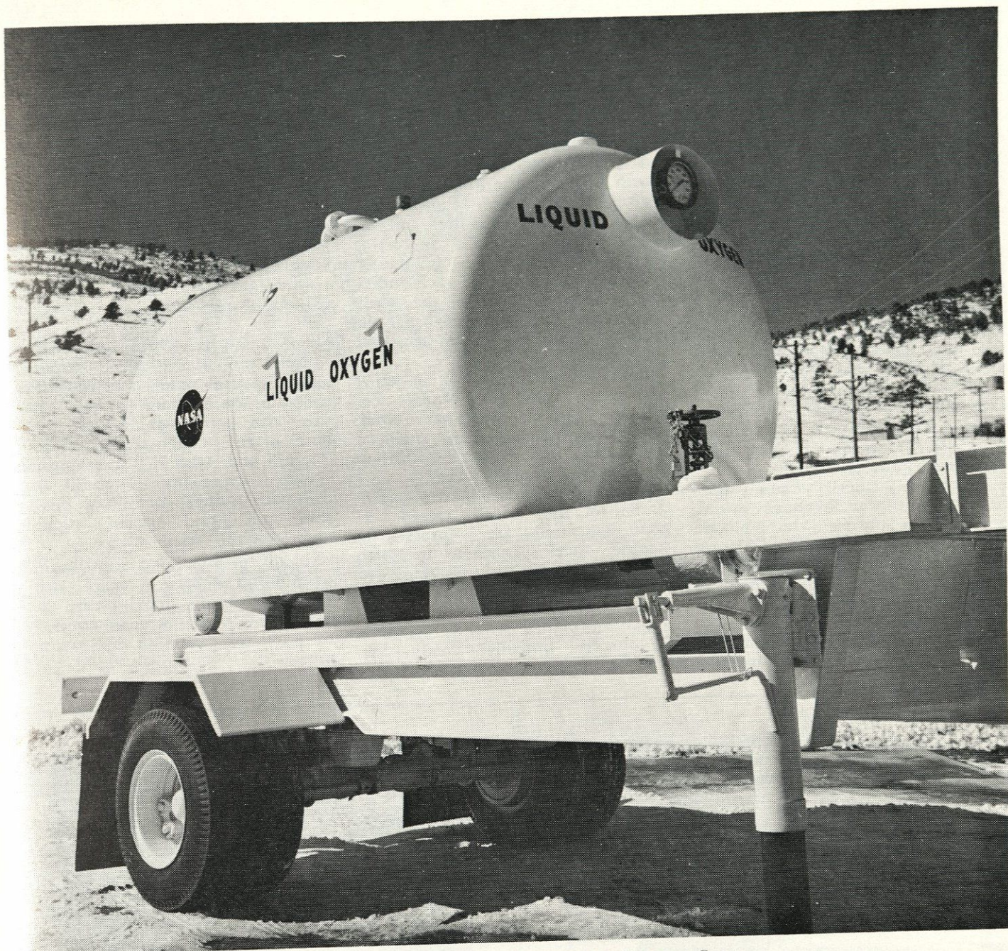
A BEECH-BUILT MOBILE STORAGE DEWAR FOR LIQUIFIED GASES
