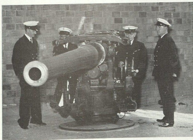
Four-inch Fifty-caliber Breech-loading Rifle, Used Principally on Submarines and Destroyers
