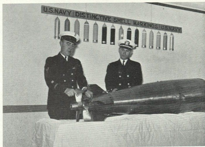
Putting Propeller Locks on the Propellers of an Eighteen-inch by Eighteen-foot Torpedo
