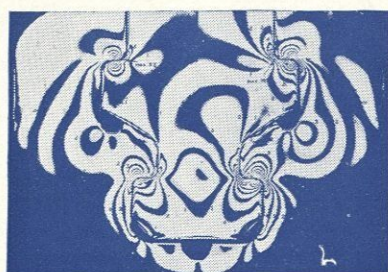
Photoelastic study of loaded turbine blade root
