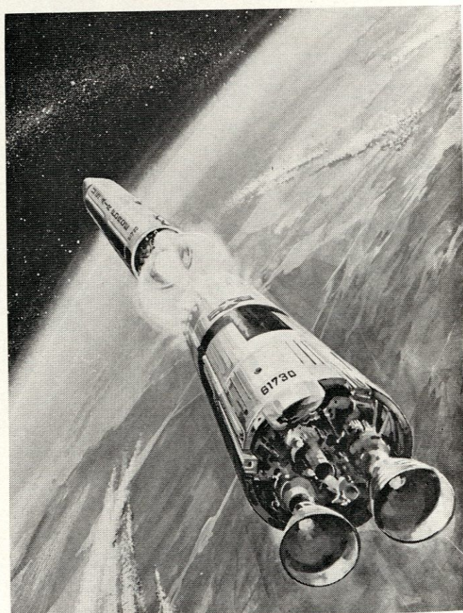
ARTIST'S IMPRESSION OF SEPARATION OF TWO STAGES AND IGNITION OF THE LAST STAGE OF TITAN II.
