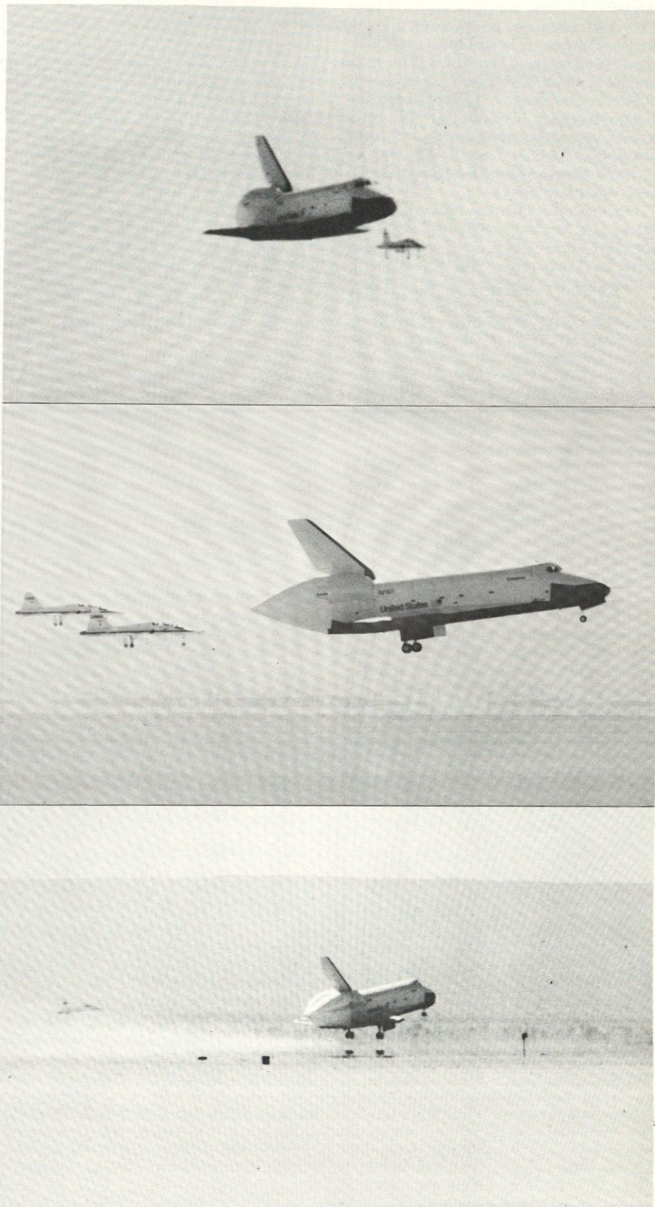
This first free flight of the orbiter took place on August 12 at Edwards AFB. The trailing vortices in the bottom picture are evidence that the Enterprise does generate some lift. Two of the five T-38 chase planes are also shown.
