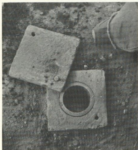
The laser alignment port on the platform assures accuracy.
