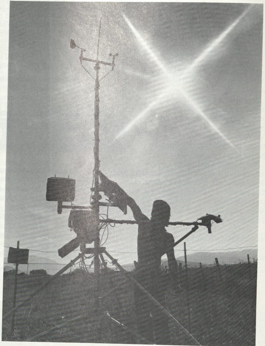
A JCEM graduate energy assistant installs one of the Center's weather stations, used to collect climatic data useful to building designers.
