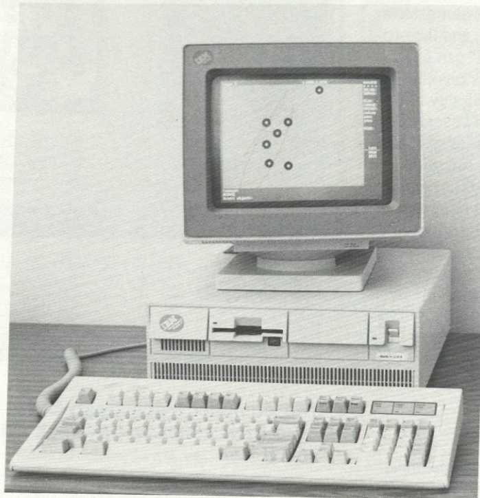
This IBM Personal System/2 Model 50 offers a high-density 3 1/2 inch floppy disk drive and a 20 megabyte hard drive.
