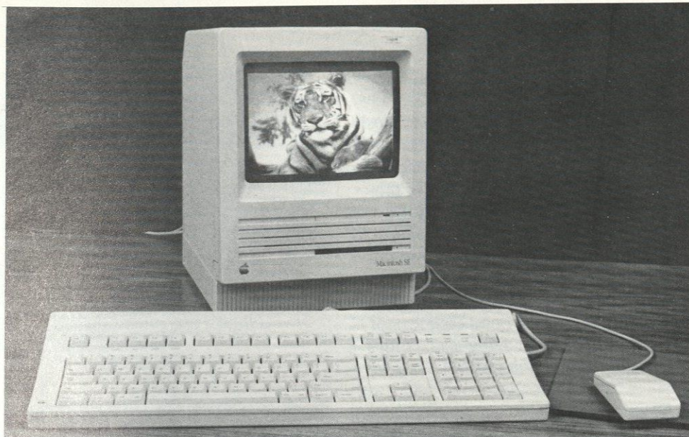
The compact Macintosh SE is shown here with 20 megabyte hard drive, 800k floppy disk drive, mouse, and extended keyboard.
