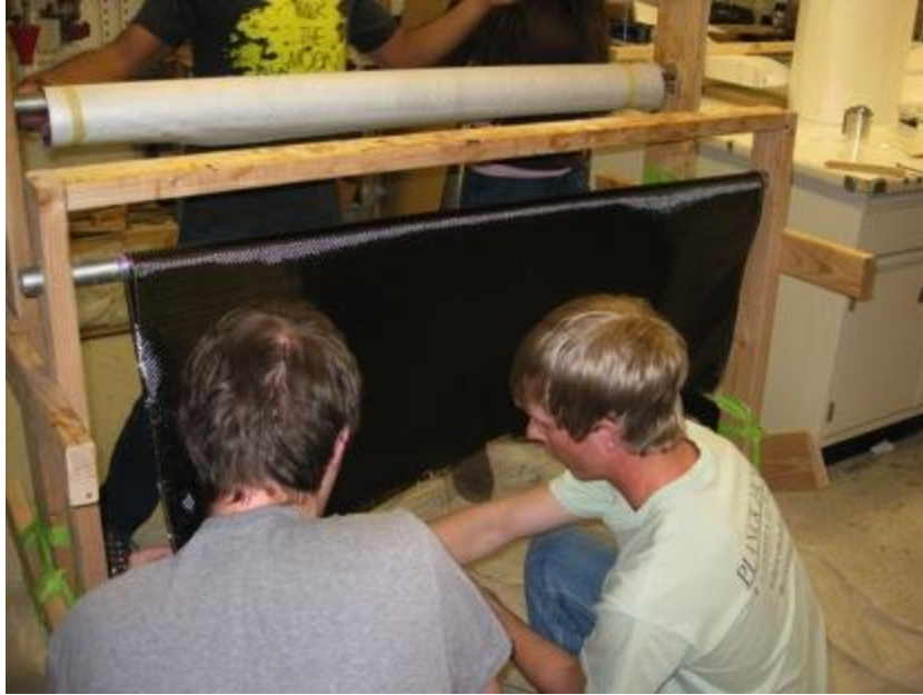
Figure 60 – The team checks the length of the carbon fiber before fabrication
