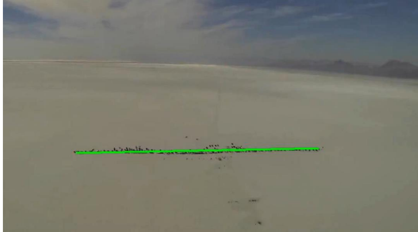
Figure 50 - Frame from Algorithm test, Green line indicates the location of the detected hazard.
