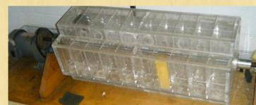
Tumbler used to mix centrifuge tubes during batch experiments
