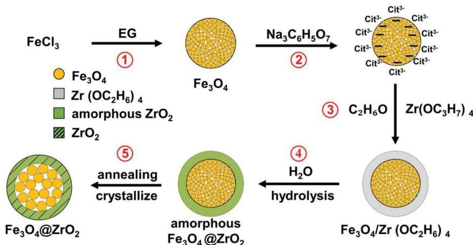
**Figure 2.** Schematic illustration of the formation processes of  $\text{Fe}_3\text{O}_4@Zr\text{O}_2$  core-shell nanocomposite (see text for details in step 1–5).
