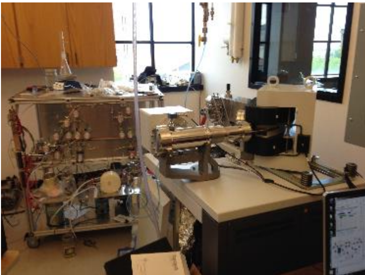
Thermo MAT253 Plus with custom designed on-line and off-line vacuum CO 2 extraction systems
