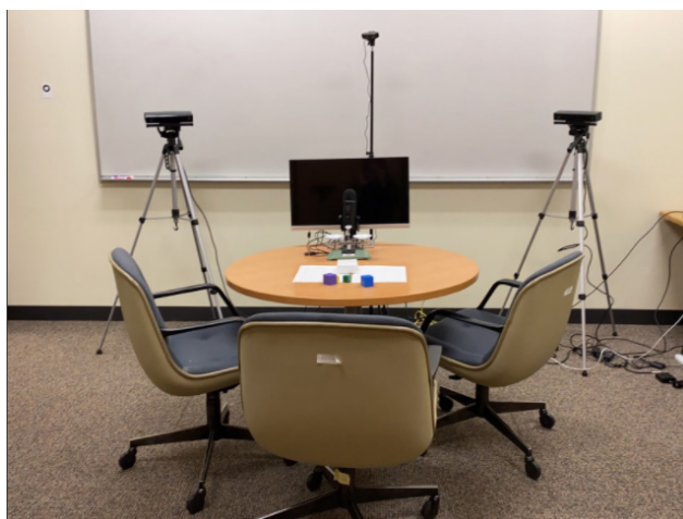
iSAT Lab setup with a webcam, Yeti mic, Kinects, and Tobii Eye Glasses.
