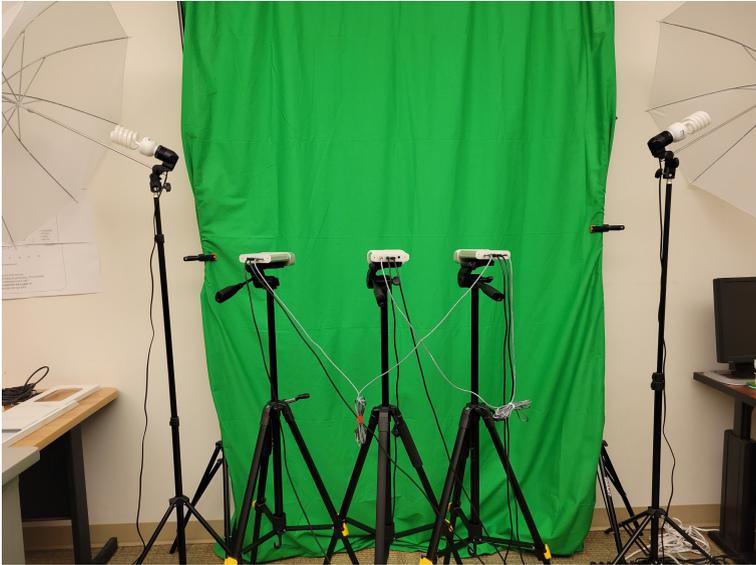
**Fig. 2.** This image represents the three Microsoft Kinect cameras with a green screen setup for real data collection. (Color figure online)
