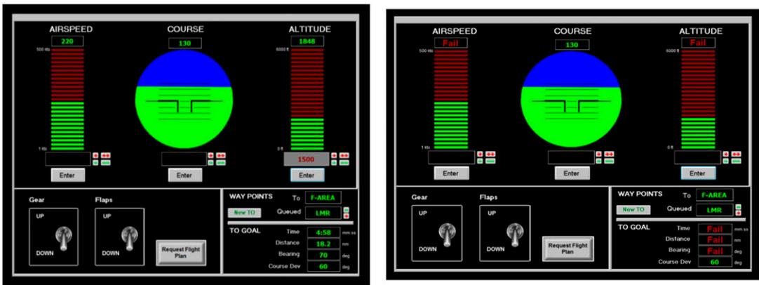
Figure 6. Example of a Type II automation failure. The left image displays the pilot's screen during normal (routine) conditions. The right image displays the failures that occurred during the Type II automation failure: The pilot cannot see Altitude and Airspeed and must obtain this information from other team members.
