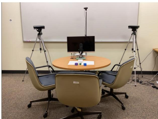
iSAT Lab setup with a webcam, Yeti mic, Kinects, and Tobii Eye Glasses.
