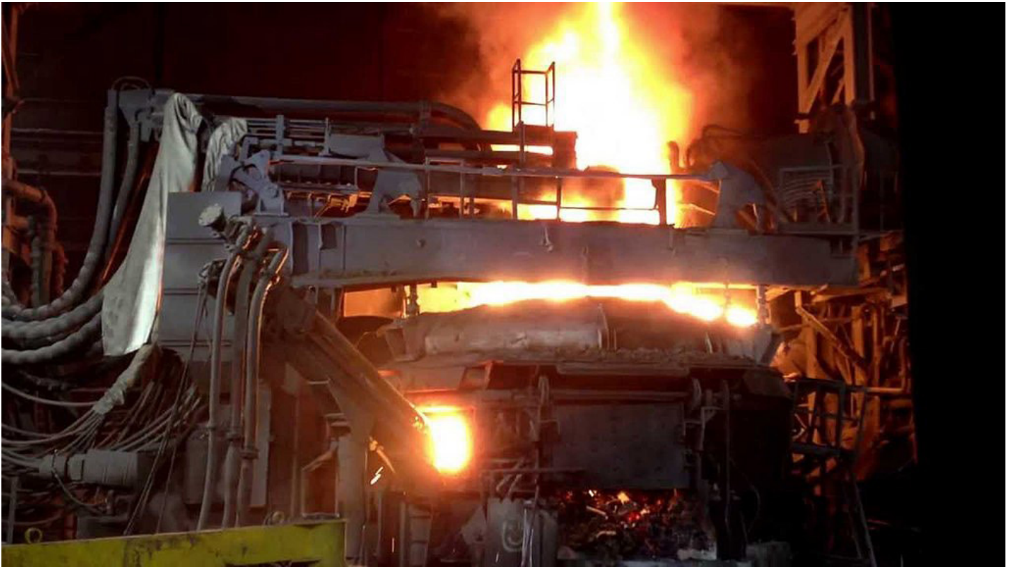
This electric-arc furnace melts steel and aluminum for rocket parts and aerospace applications at Michoud Assembly Facility, New Orleans, Louisiana. (Wikimedia Commons)
