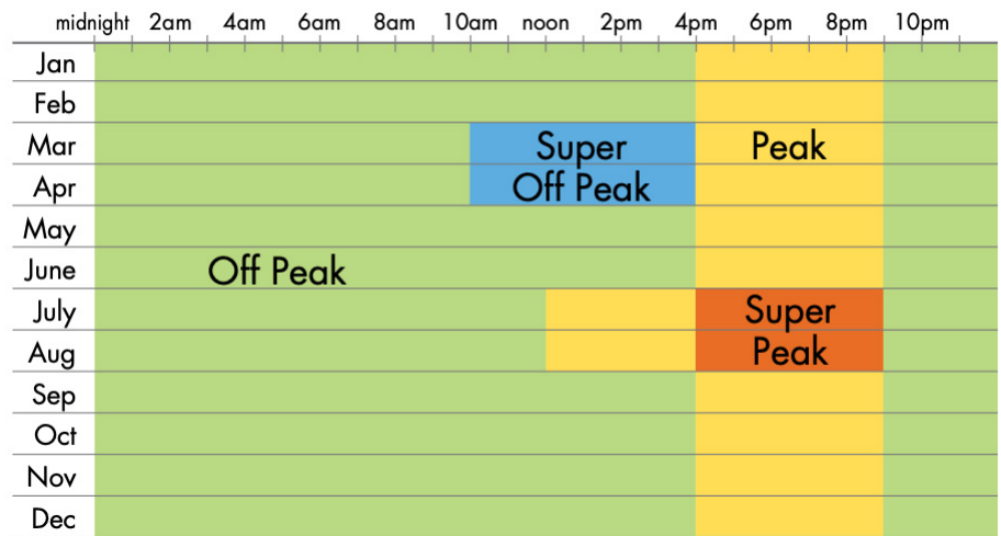
Figure 2.11. California time-of-use rates. California is rolling out optional time-of-use rate packages to all consumers, setting higher rates during peak times. (CAISO 2015)
