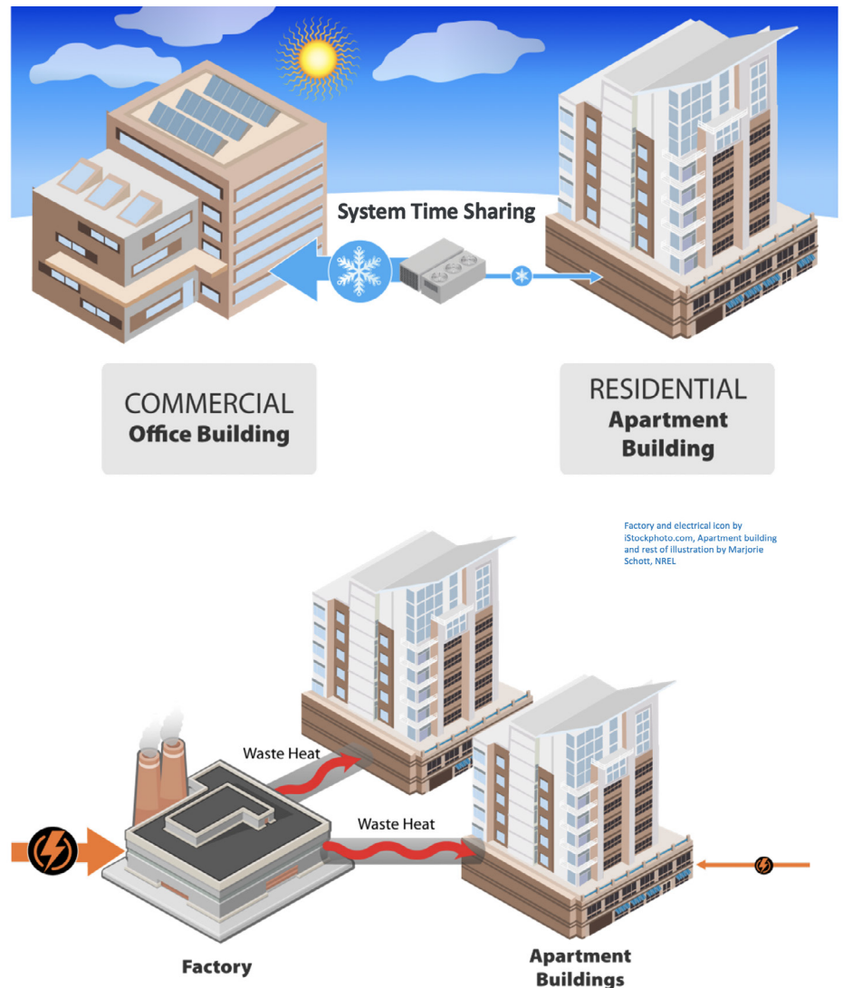
Figure 3.9. Equipment sharing in a district energy project. District energy designs can take advantage of system sharing day (top) and night (bottom). (Courtesy Marjorie Schott, NREL)
