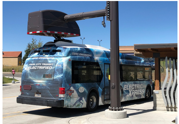
An electric bus charging station at the Kimball Junction Transit Center in Park City, Utah. (Margaret Smith / Akimeka / NREL 61251)
