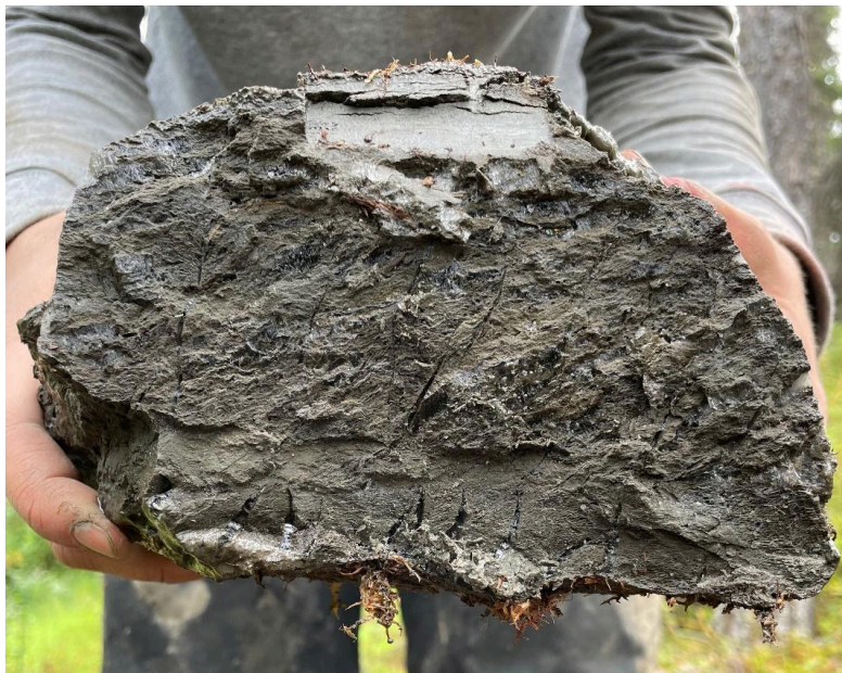
Figure 2: A block of frozen, ice-rich loess similar to those used for IRSL dating. Once excavated from the subsurface, these large chunks of loess were wrapped in foil to shield them from sunlight and transferred to a cooler to preserve their structure. They were then brought to the Luminescence Lab for processing, where we removed the outermost loess that may have been exposed to sunlight during sampling and used the inner core for IRSL analysis.
