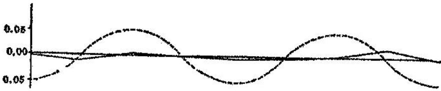
Fig. 3. Michelson's 1881 experimental result. "The dotted curve is drawn of the supposition that the displacement to be expected is one-tenth of the distance between the fringes,... From Michelson (1881)
