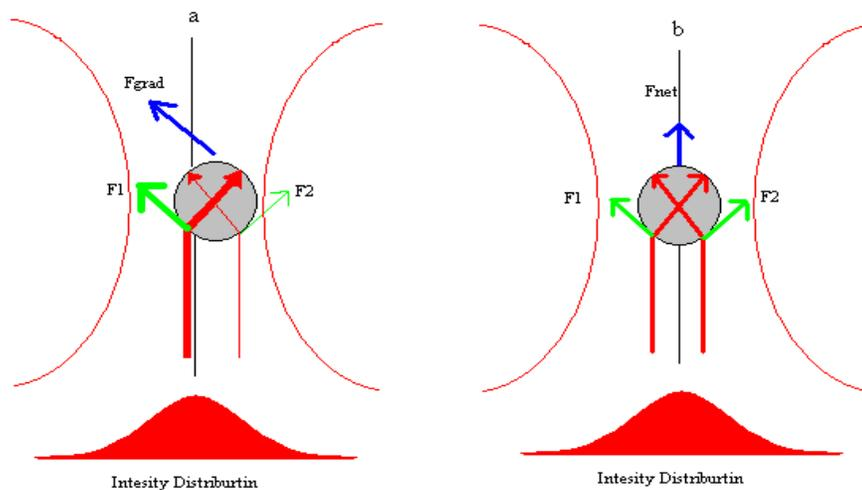
**Figure 2:** Force diagram caused by the bending of the light in the particle. (a) when the particle is not centered over the beam, and (b) when the particle is centered
