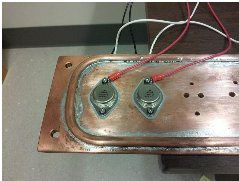
Figure 17: Water cooled FET board
