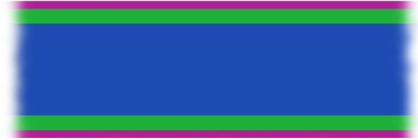
(b) Positive PR, AZ 4210, was spun onto the back and then the front of the wafer on top of the thermally-grown layers of SiO<sub>2</sub>.
