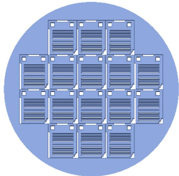
(b) This is what the wafer should look like at the completion of the KOH etch.
