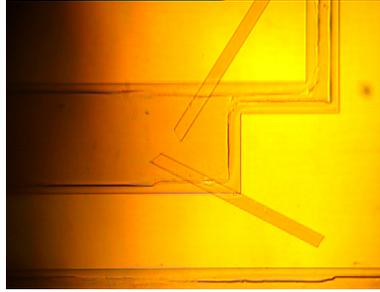
(b) This is the wafer after the BOE but before the PR was removed. Broken pieces of PR are stuck to the wafer in the wrong places.
