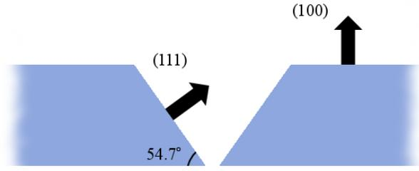
(a) This is the ideal etch geometry of a Si(100) wafer showing the (111) planes at a  $54.7^\circ$  angle with the (100) planes. The arrows drawn are normal to the surfaces of the planes.
