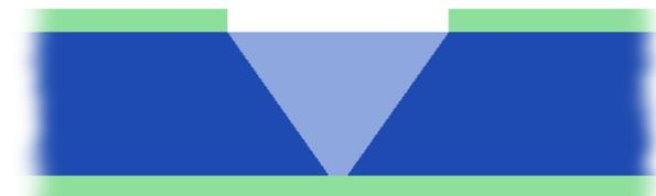
(g) Both the SiO<sub>2</sub> and Si(100) wafer were etched by the KOH solution.
