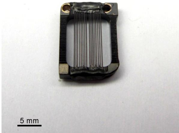
(a) This is the slit array design currently installed in the ARPES system.
