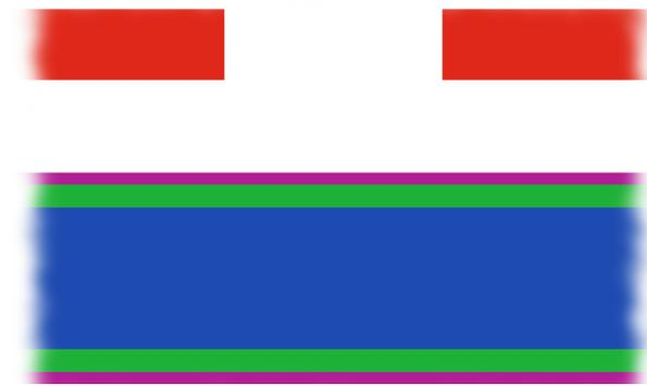
(c) This shows the mask aligned over the PR in preparation for exposure.
