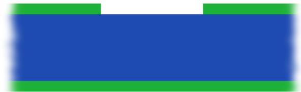
(f) The BOE created the hard SiO<sub>2</sub> mask that protected the Si(100) during the KOH etch.
