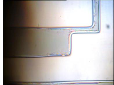
(c) This is the wafer after the BOE and after the PR was removed. The broken pieces of PR are now gone.
