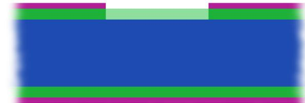
(e) The SiO<sub>2</sub> was etched where it was not protected by the PR.
