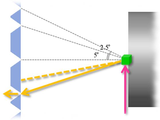
(b) This is a photograph of the current system inside ARPES with cartoons added to depict the photons (pink) striking the sample (green) which emits electrons (yellow). The electron that is deflected by the slit array (dotted yellow) is not included in the data.
