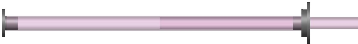
Figure 5: This is a model of the completed graphene-growth chamber with the quartz tube is shown in pink and the KFs shown in gray.
