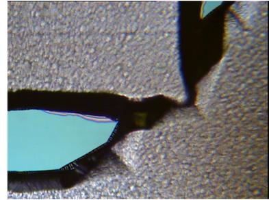
(f) After 10 hours in the KOH etch the pixelated corner feature is almost combined with the slit region.
