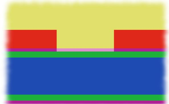
(d) The exposed PR was removed during development and protected the mask during the BOE of SiO<sub>2</sub>.
