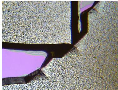
(e) After 8 hours in the KOH etch the outer corners are more rounded than square.
