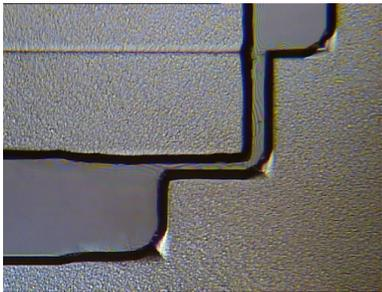
(d) After 3 hours in the KOH etch the outer corners are still recognizable.
