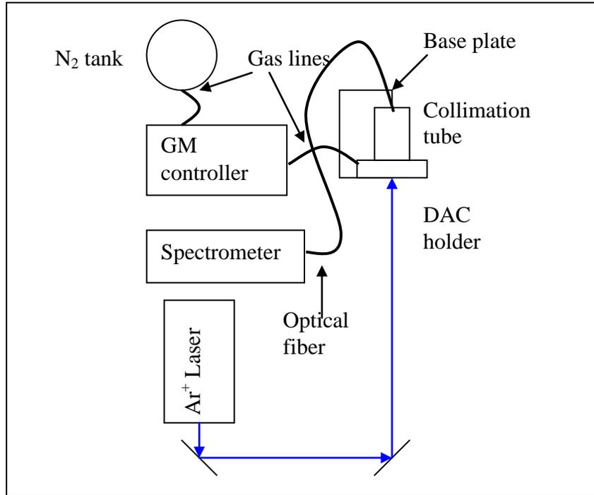
**Figure 5: Setup for absorption**
