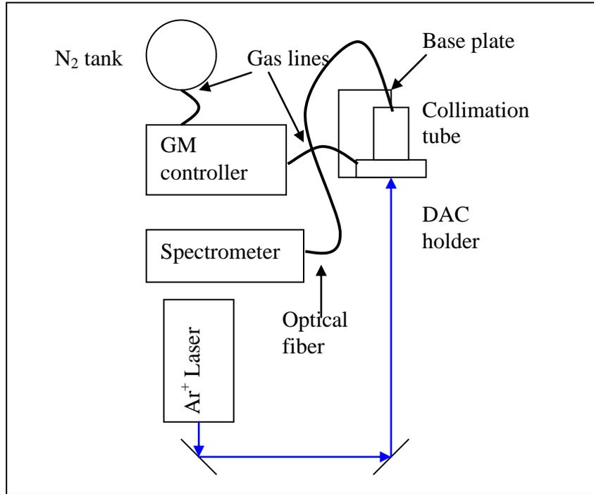
**Figure 5: Setup for absorption**
