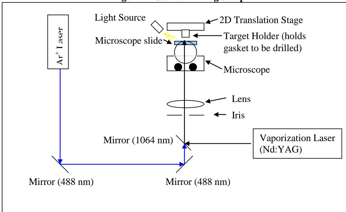
Following the beam line from the vaporization laser through to the target, the first thing encountered is a 1064 nm mirror. As the laser is reflected off of this mirror, the blue  $\text{Ar}^+$  laser is brought in from behind, and the two made collinear. The lasers then travel through an adjustable iris. Behind the iris, the beams go through a glass lens that focuses the vaporization laser down to power densities high enough to vaporize the metal of the gasket.
