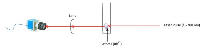
The test experiment consisted of taking Images of <sup>87</sup>Rb clouds for a variety of time-of-flight (TOF), ranging from 7 to 18 ms during the expansion period. For every TOF, three images were taken: shadow, light, and dark. A new cloud was prepared for every expansion time recorded. Figure 9 shows a sample image from the raw data.
