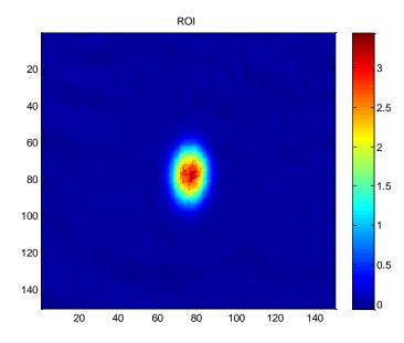
The last section of the code consists of a Gaussian surface-fitting routine. The traces at x = xcenter and y = ycenter are fit to the Gaussian surface function shown below:
