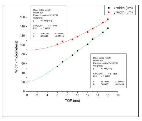
From the fitting, the velocities were found to be 8.39(5) mm/s in the x direction and 7.8(1) mm/s in the y direction. Using equation (7), the temperatures in both directions were calculated to be 0.722  $\mu$ K for x, and 0.638  $\mu$ K for y. Although the system is in thermoequilibrium, the temperatures obtained are not
