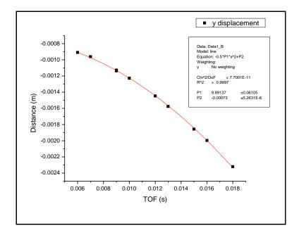
From the fitting parameters it is observed that the cloud is moving with a downward acceleration of  $9.89(6) \text{ m/s}^2$ . In other words, the cloud's acceleration is due to gravity. This result also implies that the magnification used is right.
