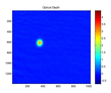
The next section of the code is designed to select a region of interest (ROI) using binned data. The OD image previously calculated was binned to increase the signal-to-noise ratio. Figure 11 shows a sample ROI image.
