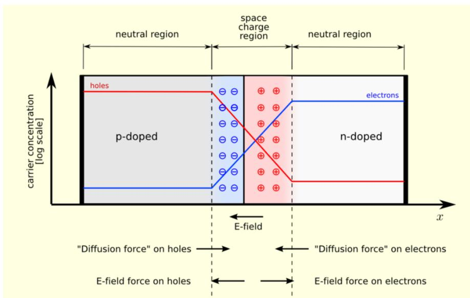
Figure 3: A simple P-N junction diagram, from <https://en.wikipedia.org/wiki/File:Pn-junction-equilibrium.png>
