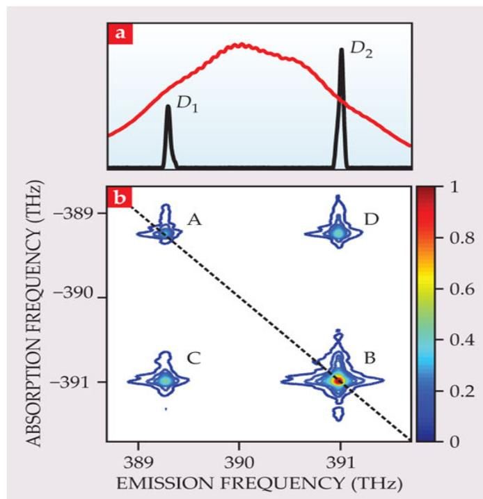
Figure 1: 1a shows the same spectrum in a more typical one-dimensional Fourier spectrum, demonstrating how much information is lost. 1b shows an example two-dimensional Fourier spectrum, where signals along the dashed line (A,B) indicate absorption and emission occur at the same frequency. The off diagonal peaks (C,D) correspond to coupling between the excited states. Figure from [4].
