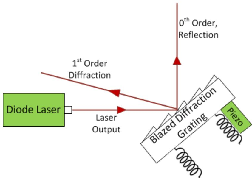
Figure 5: External cavity diode laser in the Littrow arrangement. The 1st order diffraction is not precisely aligned back into the laser cavity only for illustrative clarity. Figure 5: Laser Spectrum without the diffraction grating, demonstrating temperature tuning which was not sufficient, without measures to prevent condensation, to reach 780.2 nm. The power dependence on temperature is also easy to
