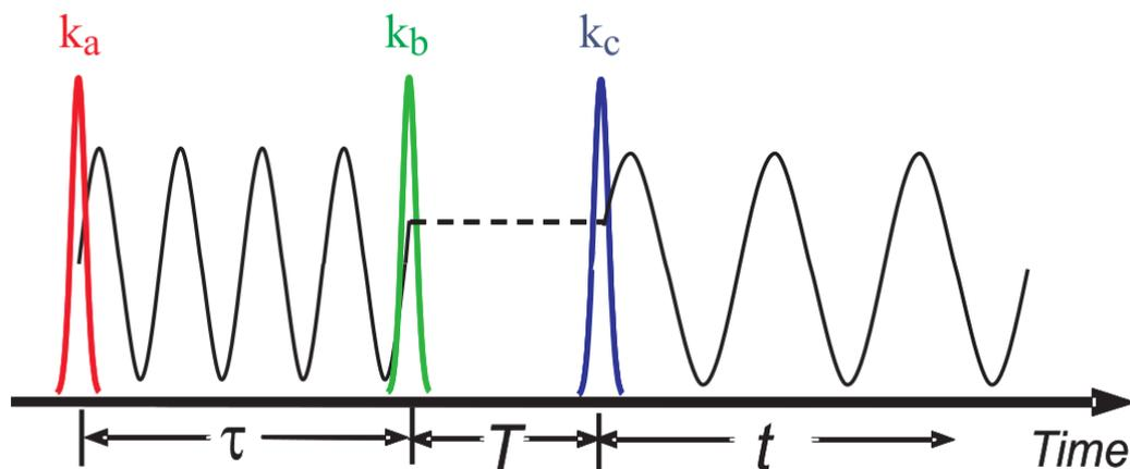
Figure 2: Illustration of pulse sequence and oscillating superpositions in 2DFT. The first pulse,  $k_a$ , creates coherence,  $k_b$  populates the system with excited states, and  $k_c$  generates a coherence that will radiate away the transient four-wave mixing signal to the spectrometer.  $T$  is typically held constant and does not appear in the final frequency correlation graph. From [5].
