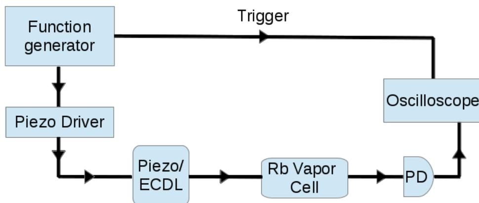
Figure 7: Electronics setup. Current and temperature controller not shown, but can be considered part of the laser system. "PD" indicates the photodiode, while arrows indicated the direction signals travel.
