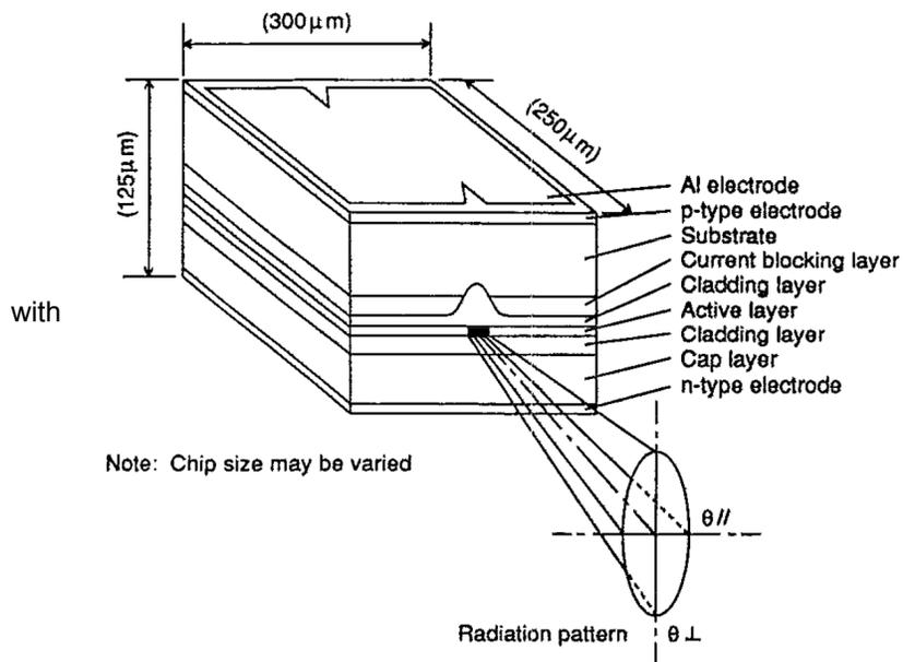
Figure 4: Simple diagram of a diode laser, illustration of the elliptical beam divergence. From [2].
