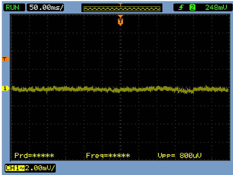
Figure 9: Oscilloscope screenshot of the photodiode noise, with the DC signal subtracted away.
