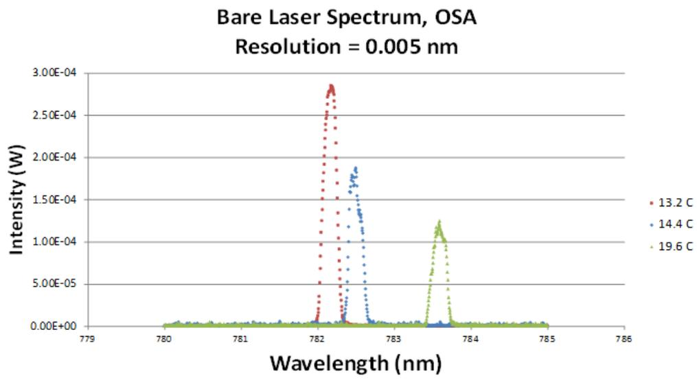
Figure 6: Laser Spectrum without the diffraction grating, demonstrating temperature tuning which was not sufficient, without measures to prevent condensation, to reach 780.2 nm. The power dependence on temperature is also easy to observe.
