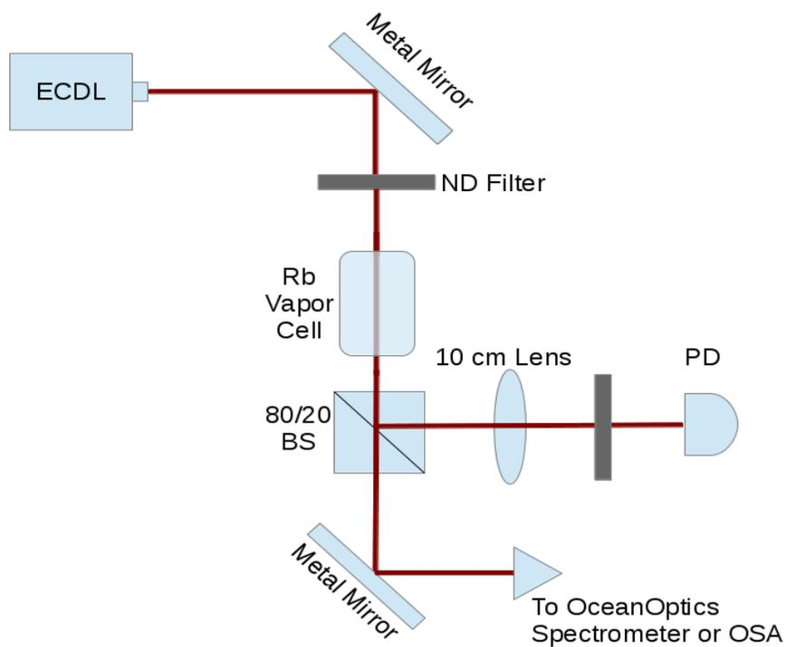
Figure 8: A diagram of the optics in the beampath for my experiment.
