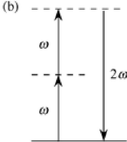
Figure 2: Energy level diagram describing the SHG process. Reproduced from Boyd. [5]
