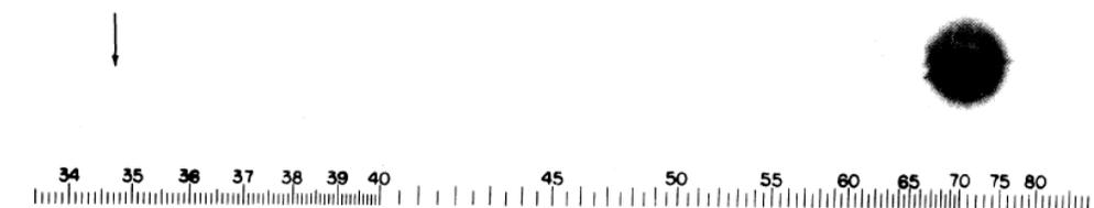
Figure 1: The first image of a second harmonic signal, generated by focusing a ruby laser on crystalline quartz. The second harmonic signal which should be visible at 347nm has been removed. [1]
