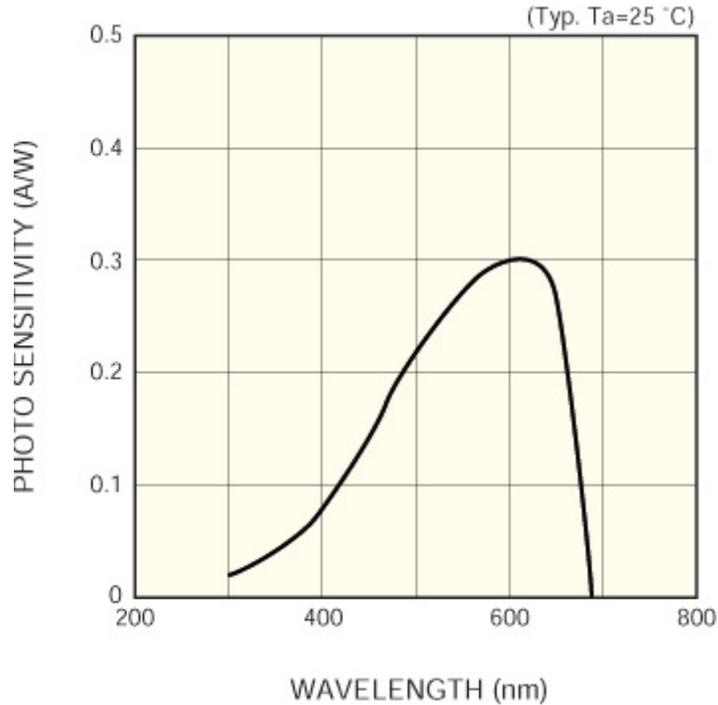
Figure 8: Photosensitivity of GaAsP, peaking at 640nm before falling off completely just before 700 nm. [13]
