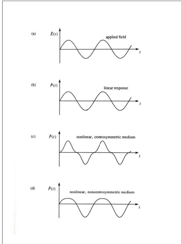
Figure 3: Optical response of charge distribution of a dielectric in an applied sinusoidal electric field (a) that induces a linear polarization (b) and a nonlinear polarization that is dependent on the particular crystal symmetry of the medium (c), (d). Reproduced from Boyd. [5]
