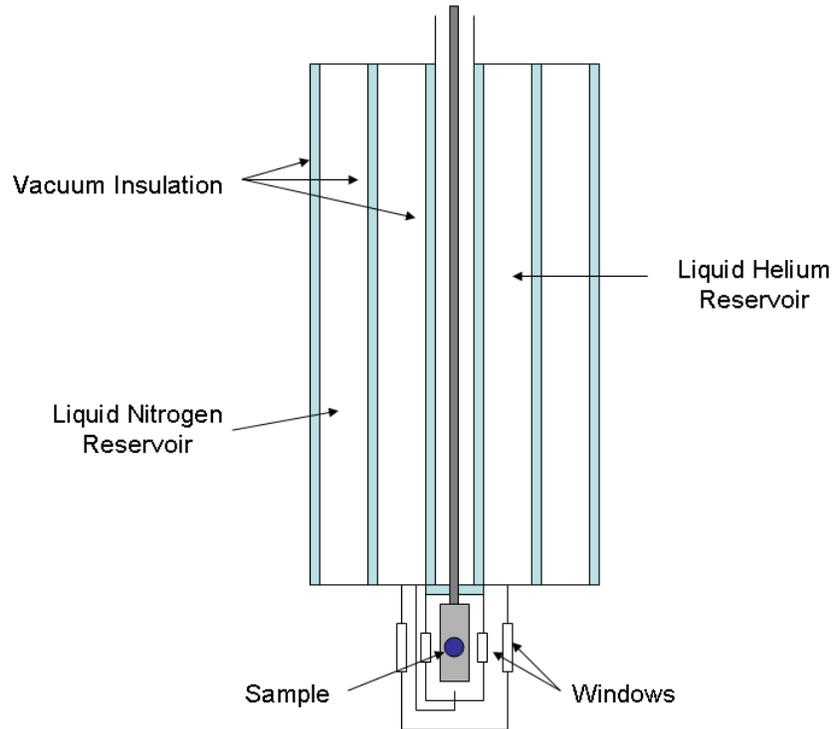
Figure 9: A simplified schematic of the CRYO Industries model 8CN Optical Cryostat.
