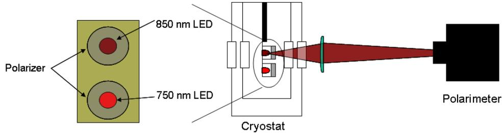
Figure 10: Basic setup of the window characterization experiment.
