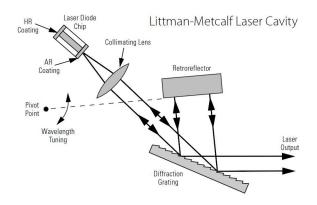
Figure 2. Diagram of Vortex laser cavity [4]
