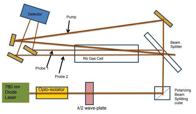
Figure 3. Optical set-up for Doppler free saturated absorption spectroscopy
