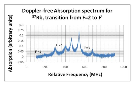
Figure 5. This shows the Doppler-free absorption spectrum of the <sup>87</sup>Rb transition between the  $5^{2}S_{1/2}$  and  $5^{2}P_{3/2}$  states from P =
