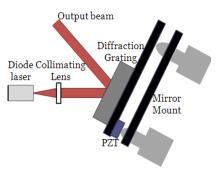
Figure 1. This figure shows the arrangement of the components of the tunable diode laser. These components are mounted on a baseplate, and then enclosed in an aluminum box.
