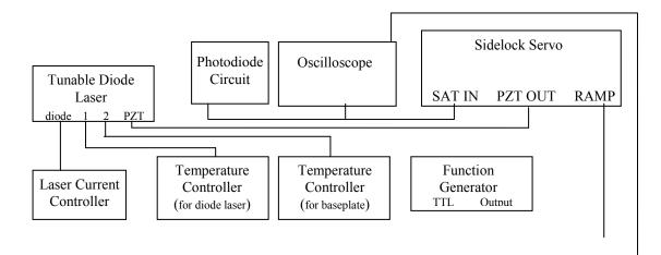
Figure 3. This shows the final arrangement of the electrical equipment needed for the tunable diode laser, saturated absorption spectroscopy, and locking to the side of an absorption peak. Note that the power and current supplies needed to run the equipment are not shown.
