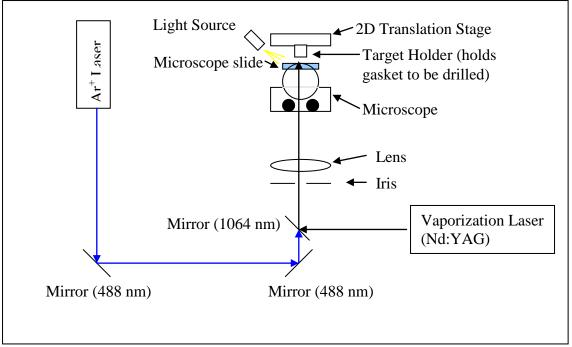
Figure 2: Gasket Drilling Setup
