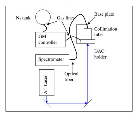
**Figure 4: Setup for fluorescence**
