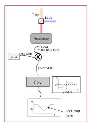
Figure 7- Diagram of beat mechanism
