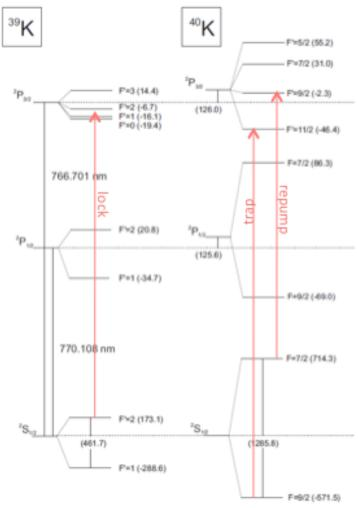
Figure 3- Fine and hyperfine structures of <sup>39</sup>K and <sup>40</sup>K including transitions utilized in creating a MOT<sup>1</sup>
