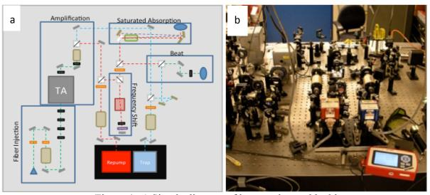
Figure 4- a) Simple diagram of laser tuning and locking configuration, b) Actual picture of lab apparatus
