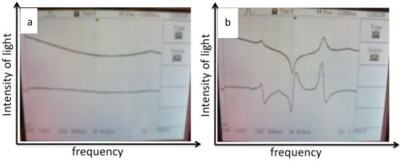
Figure 6- a) Signal from a single 767nm laser passing through a Potassium cell b) Signal from two counter propagating 767nm lasers, which overlap in the Potassium cell
