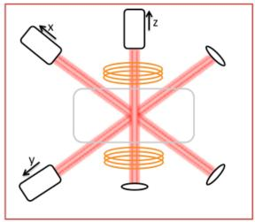
Figure 1- Simplified diagram of a MOT chamber
