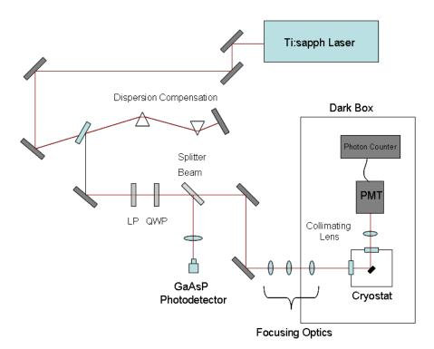
Figure 7: The purposed experimental setup.
