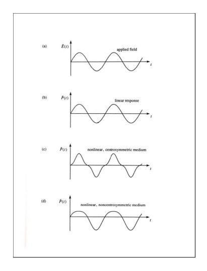
Figure 3: Optical response of charge distribution of a dielectric in an applied sinusoidal electric field (a) that induces a linear polarization (b) and a nonlinear polarization that is dependent on the particular crystal symmetry of the medium (c), (d). Reproduced from Boyd. [5]
