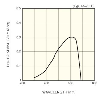
Figure 8: Photosensitivity of GaAsP, peaking at 640nm before falling off completely just before 700 nm. [13]
