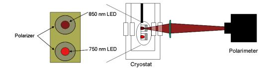
Figure 10: Basic setup of the window characterization experiment.
