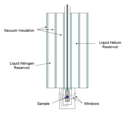
Figure 9: A simplified schematic of the CRYO Industries model 8CN Optical Cryostat.
