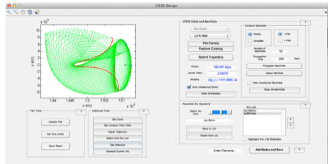
Fig. 13. SEL2 manifold surface (green) propagated in ATD with selected trajectory (red).
