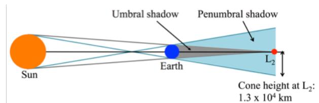
**Fig. 12.** Translation of Earth shadow avoidance requirement to maximum cone angle constraint.
