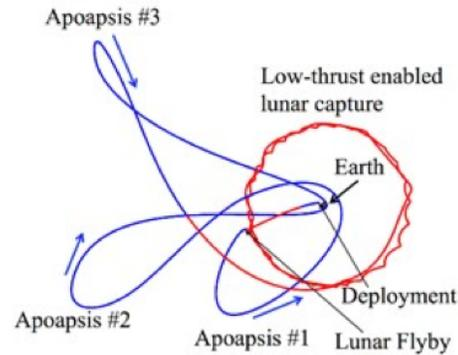
Fig. 7. Sample Lunar IceCube trajectory design in the Sun-Earth rotating frame within an ephemeris model including natural (blue) and low-thrust (red) arcs.
