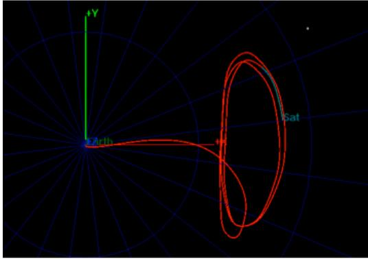
**Fig. 15.** Transfer trajectory propagated and differentially corrected in GMAT.
