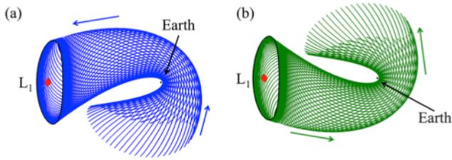
**Fig. 8.** (a) Stable and (b) unstable manifolds generated in ATD for Lunar IceCube transfer trajectory design.
