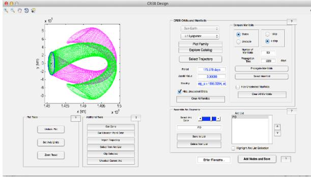
**Fig. 1.** ATD graphical interface with user-generated stable (green) and unstable (magenta) Sun-Earth  $L_1$  Lyapunov manifolds.
