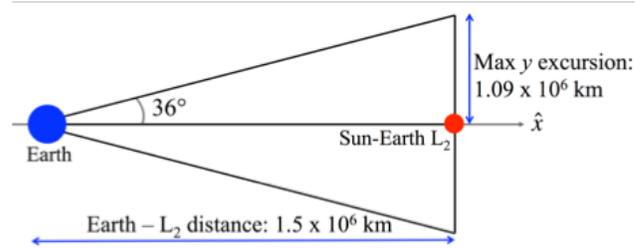
**Fig. 11.** Translation of maximum SEL2V angle requirement to constraint on  $y$ -amplitude of libration point orbit in the Sun-Earth rotating frame.
