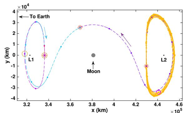
**Fig. 7.** Constraints are enforced during corrections: two state constraints (gold circles) to preserve  $L_1$  halo periodicity, one Jacobi Constant constraint to preserve the  $L_2$  quasi-halo (magenta circle), and three maneuver locations (red asterisks)
