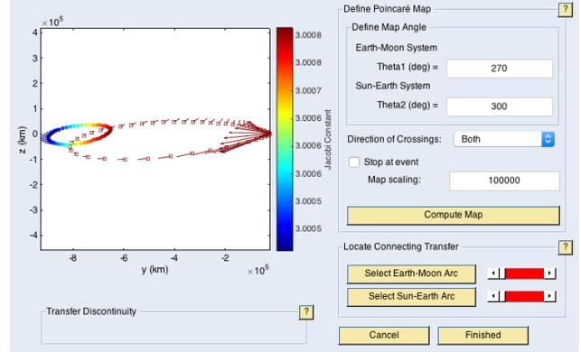
**Fig. 13.** Poincaré mapping tool to facilitate the identification of links between Earth-Moon and Sun-Earth manifold arcs
