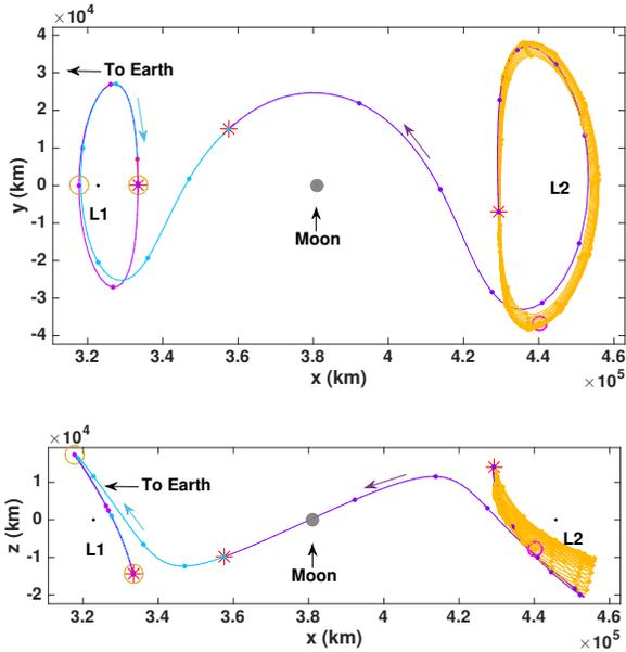
**Fig. 8.** A corrected transfer in the Earth-Moon CR3BP with a total  $\Delta V$  of 39 m/s including an  $xy$ -projection (top) and  $xz$ -projection (bottom)
