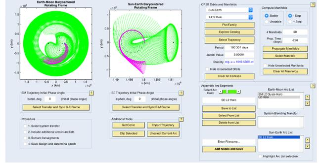
**Fig. 11.** System Blending Module: Unstable manifolds (magenta) emanate from an Earth-Moon  $L_2$  halo orbit and flow into stable manifolds (green) that asymptotically approach a Sun-Earth  $L_2$  halo orbit
