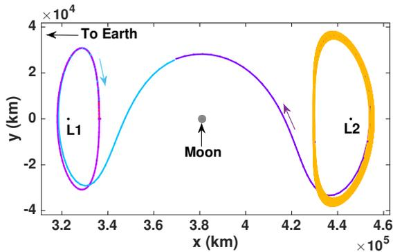
**Fig. 5.** An end-to-end, initial transfer design between an Earth-Moon  $L_2$  quasi-halo structure (gold) and an  $L_1$  halo orbit (magenta), represented in the Earth-Moon rotating frame
