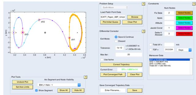
**Fig. 6.** CR3BP Corrections module: The discretized transfer design is decomposed into individual segments (colored lines), each beginning at a node (colored dots). The interface supplies tools to constrain nodes and adjust the corrections algorithm's settings
