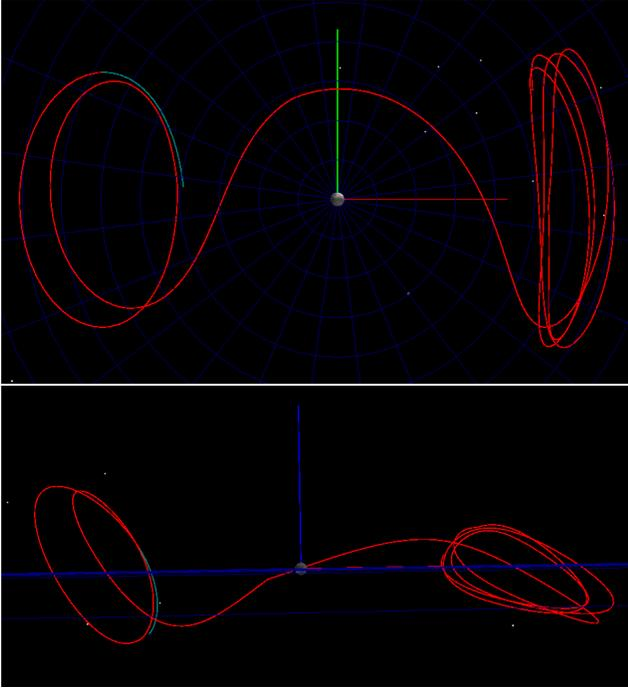
**Fig. 10.** Trajectory in GMAT:  $xy$ -projection (top) and  $xz$ -projection (bottom), Earth-Moon rotating coordinates
