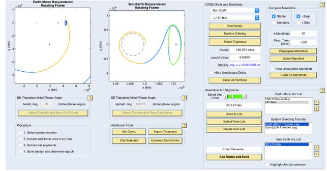
**Fig. 15.** An end-to-end transfer from an Earth-Moon  $L_2$  quasi-halo structure to a Sun-Earth  $L_2$  halo orbit.
