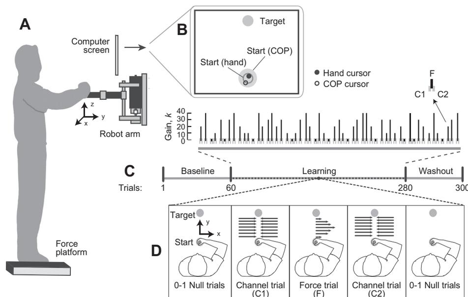
Fig. 1. *A*: apparatus. *B*: visual feedback provided to subjects on computer screen. *C*: experimental protocol and sample trial list. Each black line represents a force trial of a specified gain; each pair of channel trials is represented by the pair of short gray lines bracketing each force trial. *D*: example trial triplet, illustrating forward (+y) reaching movements and rightward (+x) perturbing forces (force trials). COP, center of pressure.
