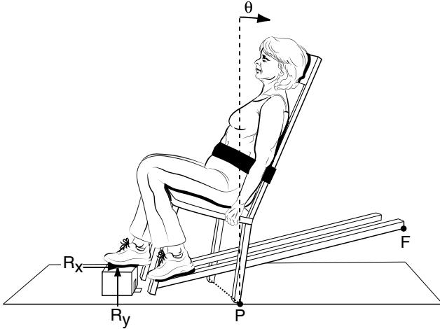
Fig. 2. Schematic of a subject starting her attempt to balance over line 'P' by varying the unipedal reaction forces  $R_x$  and  $R_y$ . A 20 cm-wide waist belt was used to strap the subject to the chair for safety.
