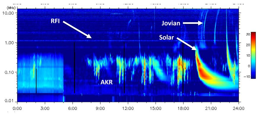
The WAVES instrument on the Wind spacecraft at Solar-Earth L1 shows solar radio bursts, Earth's auroral radio bursts (AKR), terrestrial ground-based transmitters (RFI), and Jovian radio emissions, during the 24 hr interval of 2/20/2012. ROLSES could do the same.
