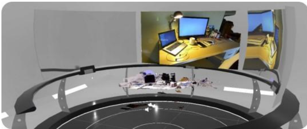
Figure 9: This prototype innovatively unifies concepts from both cyber-physical and virtual control room paradigms that are needed to deploy radio telescopes and explore the Moon. It provides users with egocentric (live stereoscopic video stream) and exocentric (3D environmental reconstruction) information to enhance detail and overall situational awareness.
