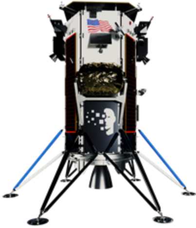
Figure 4: The CLPS IM-1 NOVA-C lander will carry the ROLSES low radio frequency payload to the South Pole in 2023 setting the stage for subsequent CLPS Dark Ages 21-cm observations in 2025. Measurements will include the surface plasma sheath and lofted dust, the lunar subsurface, and the Galactic foreground. Credit: Intuitive Machines.
