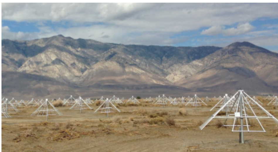
Figure 6. Looking east from the center of OVRO-LWA, a dipole array in California operating at sub-100 MHz frequencies that images the entire viewable hemisphere to simultaneously monitor thousands of stellar systems in search of stellar and planetary radio emission.
