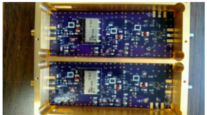
Figure 1: Photo of the initial DAPPER/CTP prototype receiver module. Full dual polarization version with noise calibration was assembled and is ready for correlation tests.
