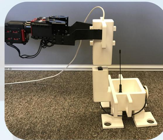
Fig. 4: Robotic arm completing connection to power antenna.
