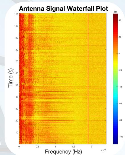
Fig. 5: The waterfall plot is a graph of time vs. frequency of the signal with power depicted in color.
