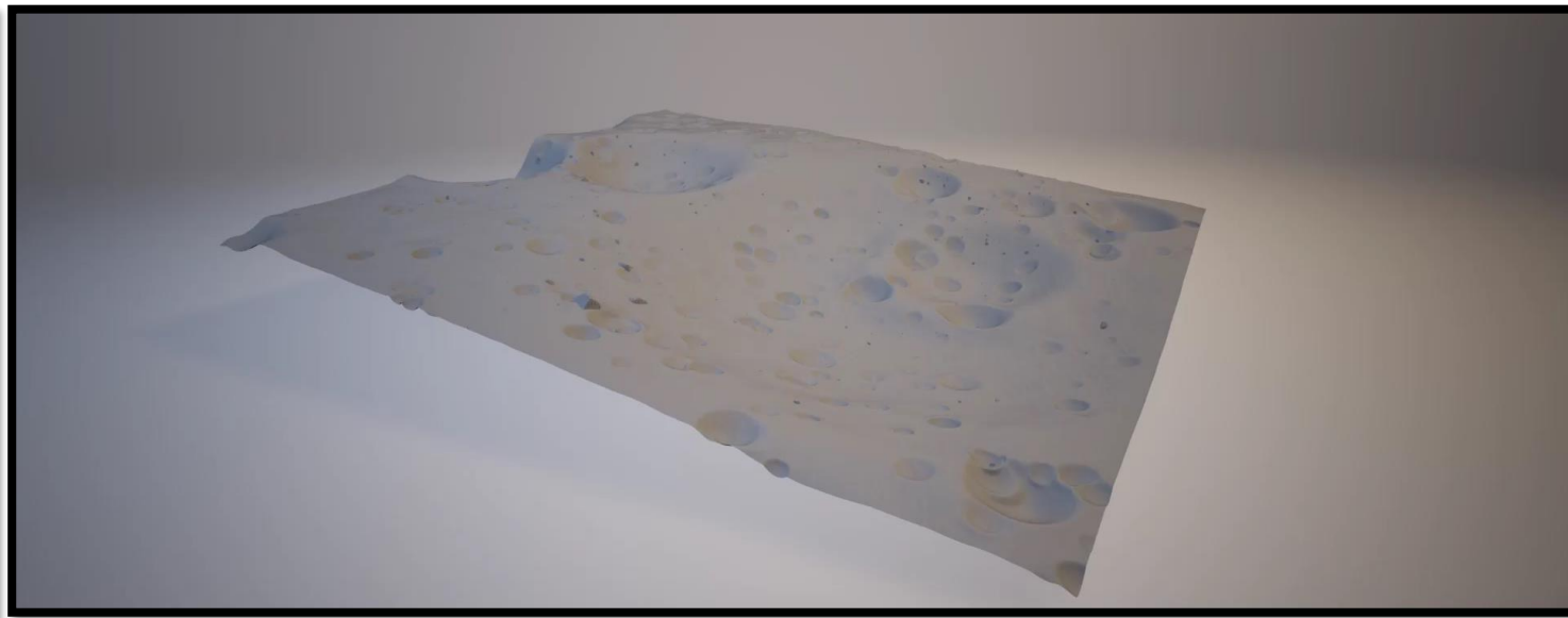
1 km x 1 km area near the Hermite A crater, located near the north pole of the Moon. The synthetic digital elevation model is based on publicly available images and laser altimetry of the Hermite A region that were acquired with LRO. Thanks to T. Fong.
