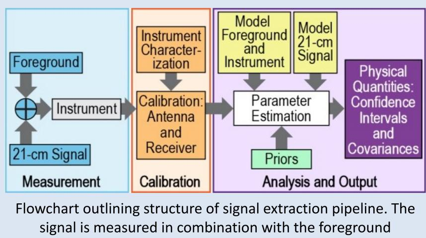
through the instrument. The data is then calibrated before parameter estimation is performed. For more details on the pipeline, see Burns et al. (2017) and the companion poster by Rapetti et al.
