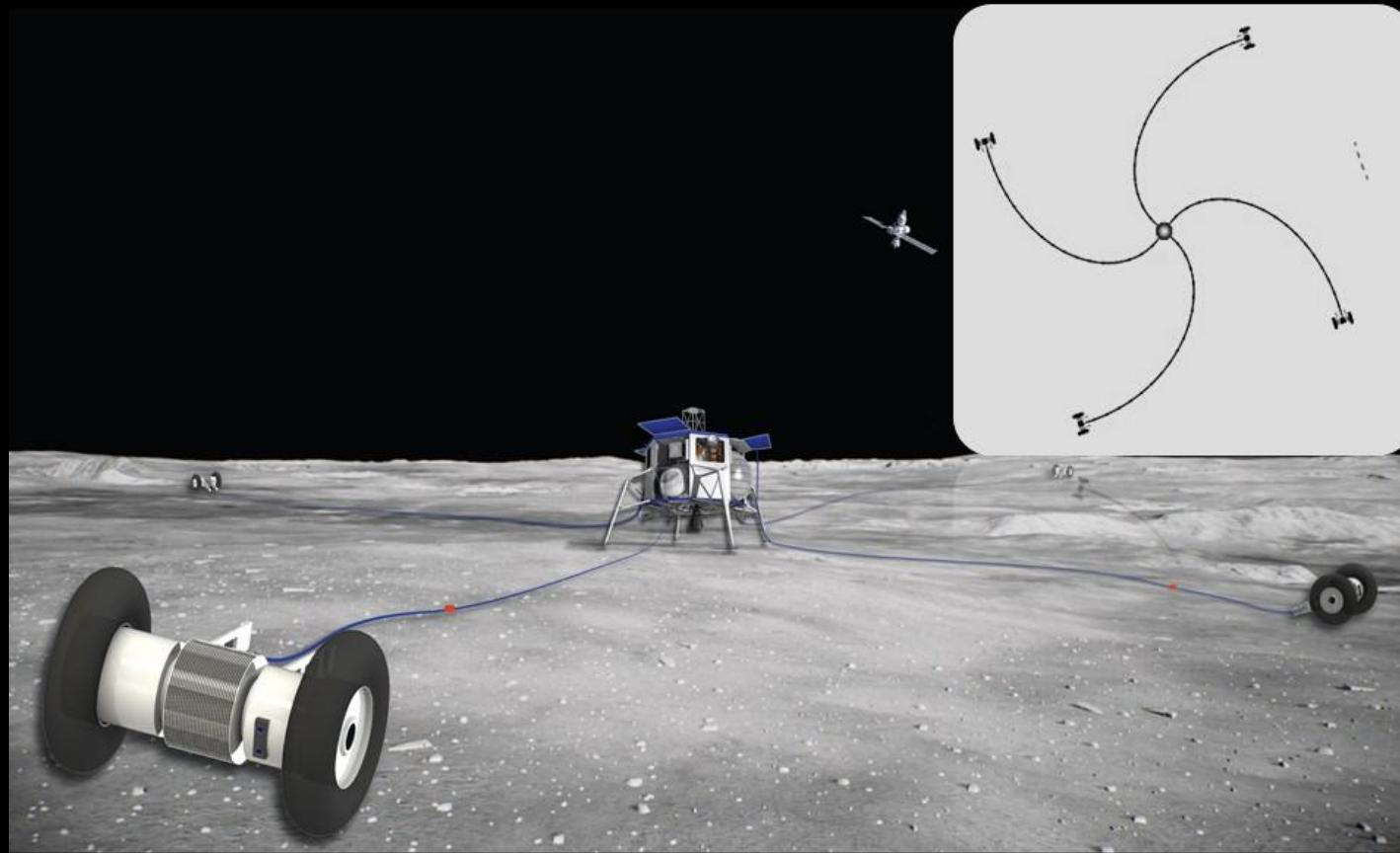
FARSIDE consists of three components: a commercial lander carrying the base station, four single-axel rovers to deploy antenna nodes, and a 128x2 (two orthogonal polarizations) node antenna array.
