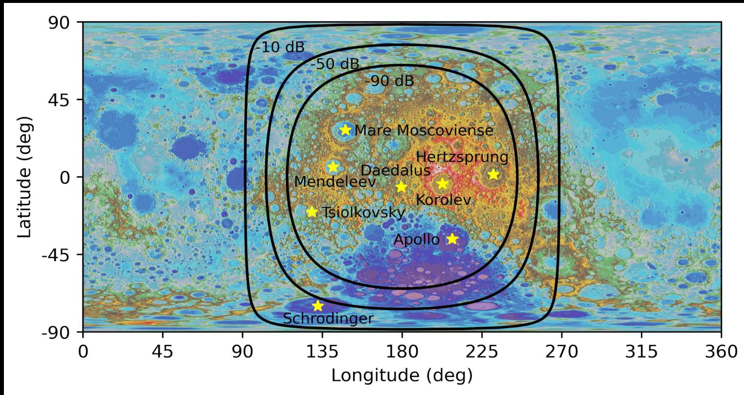
Map of RFI suppression at 100 kHz based on numerical simulations from Bassett et al. (2020). Contours indicate suppression of -10, -50, and -90 dB relative to the incident intensity. Map colors indicate elevation. Potential landing sites are indicated by the yellow stars.
