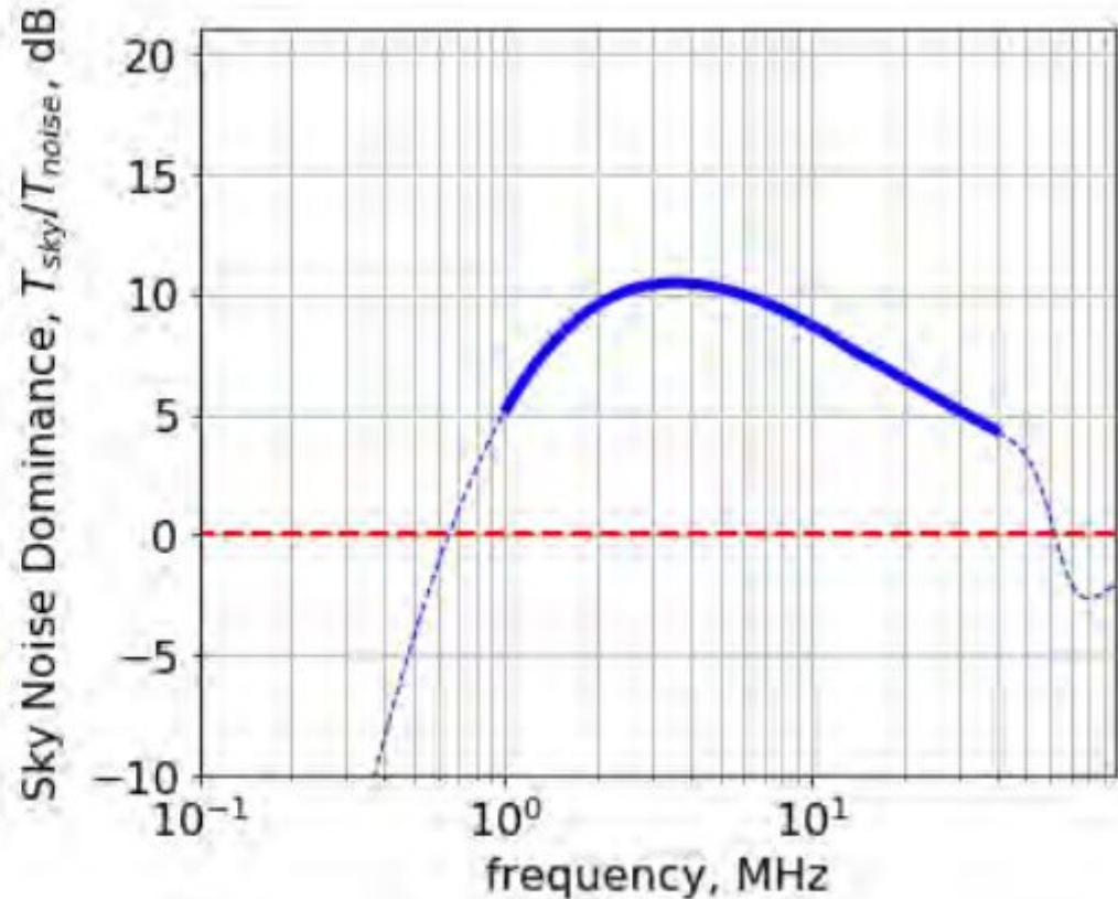
**Figure 3.5-1.** Sky noise dominance as a function of frequency are shown for the low band (*left*) and high band (*right*) antennas. The red dashed line at 0 dB indicates where sky noise would be equal to other sources of noise. The band of operation is shown as a thick line for each case.
