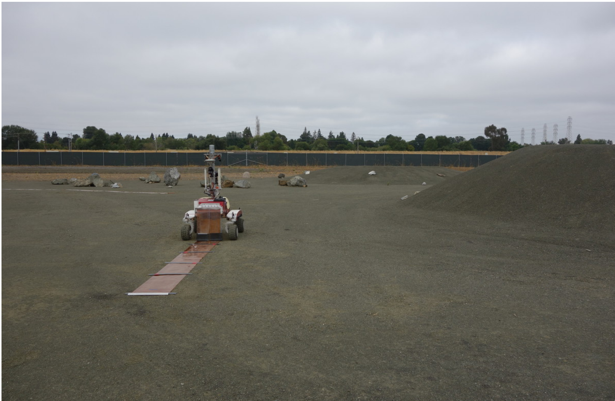
Crew Session #2 – K10 deploying simulated polyme antenna under the supervision of Luca Parmitano on ISS (2013-07-26)
