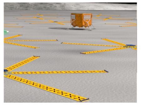
Dipoles (1x1 m) on Kapton 1500 dipoles/station DALI: 300 stations ROLSS: 1 station
