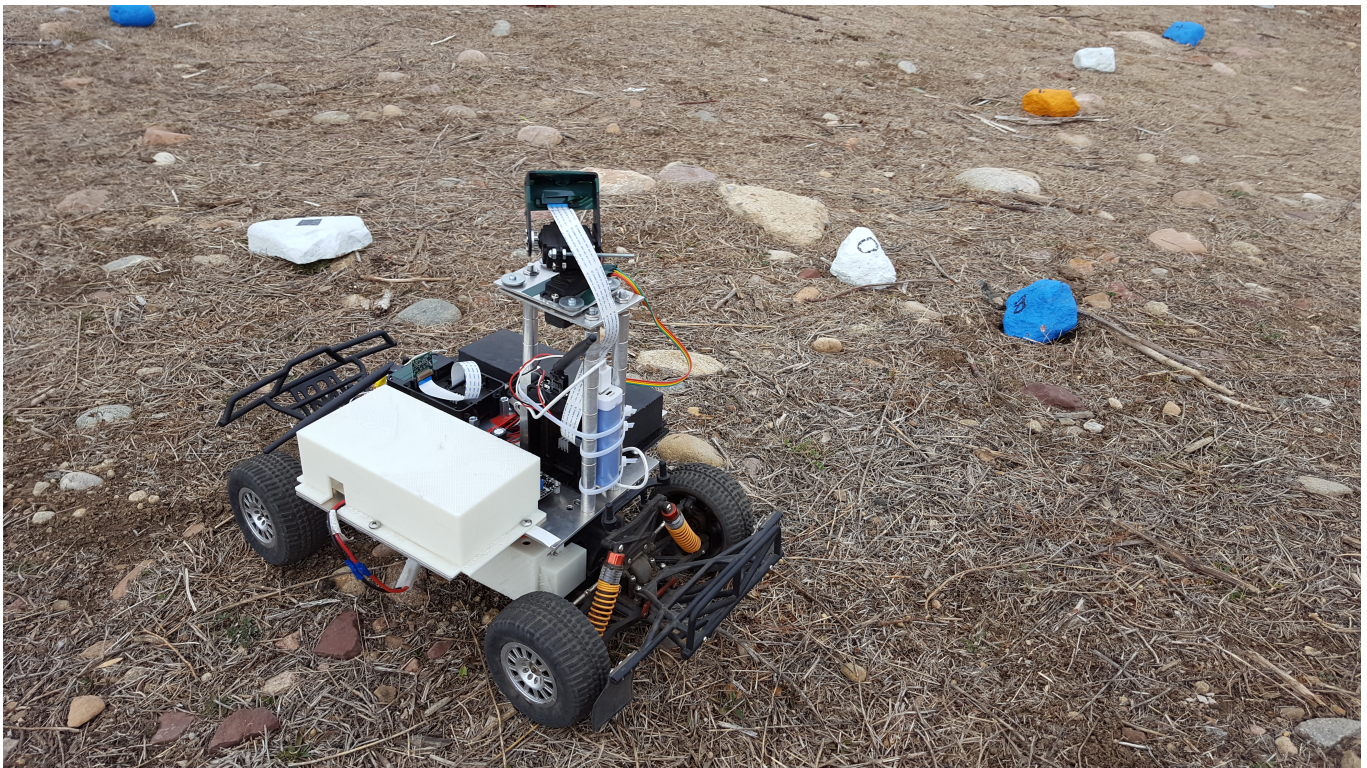
Figure 2: Close up view of the student-built COTS rover at the University of Colorado Boulder. The forward facing stationary camera is mounted at the front and the top camera is mounted on two servos for manipulation. The various electronics controlling the rover are housed underneath the white and black protective shields. The painted rocks are exploration targets for this teleoperated rover.
